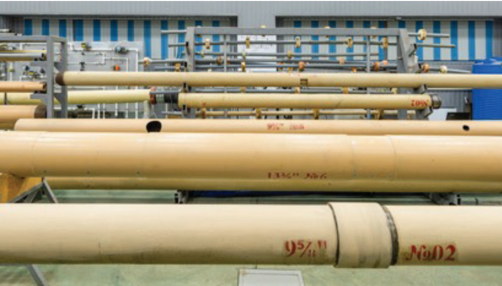
Pulse testing lab comprises various size tubing/casings with and without defects into which the Pulse tool is placed for rigorous testing.
